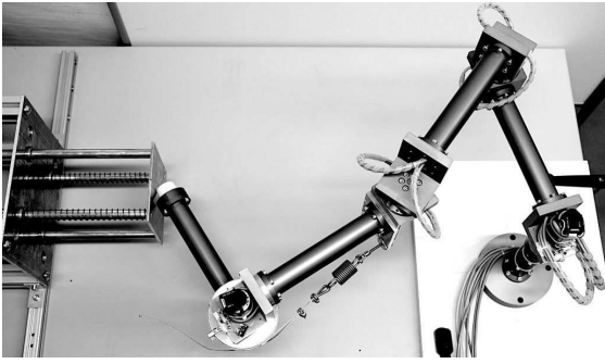
Fig. 1. Top view of the experimental setup. The ViSHaRD4 arm is shown together with the spring loaded plate.
