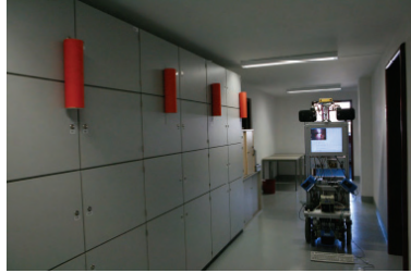
Fig. 3.4. Experiment scenario using ACE and four artificial landmarks
