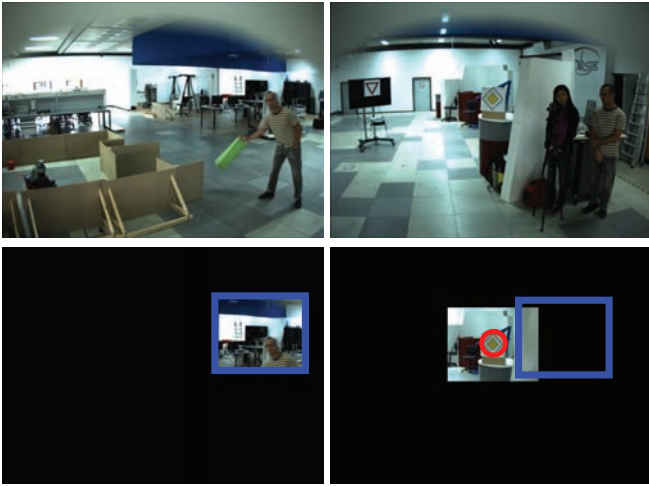
Fig. 3. Left column: attention selection in bottom-up state; Right column: attention selection in top-down state; Top row: original input images; Bottom row: the resultant images; Rectangle in solid lines: the salient/surprising image region; Masked region: the current focus of attention; Circle: detected target object.
