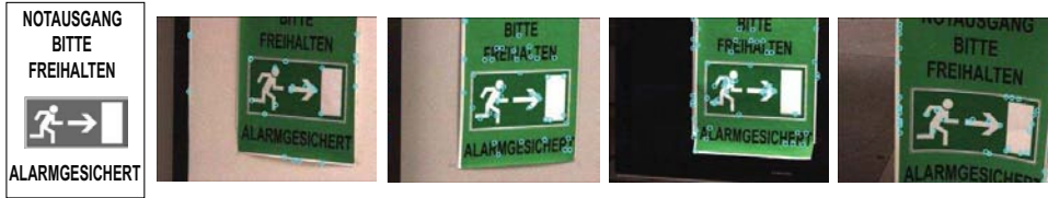
Fig. 6. The sample image of the target object used in the experiment (left) and four images of the target objects captured by the high-resolution telephoto camera during the experiment using B1T1K1. Blue circles: the matched SIFT feature points.
