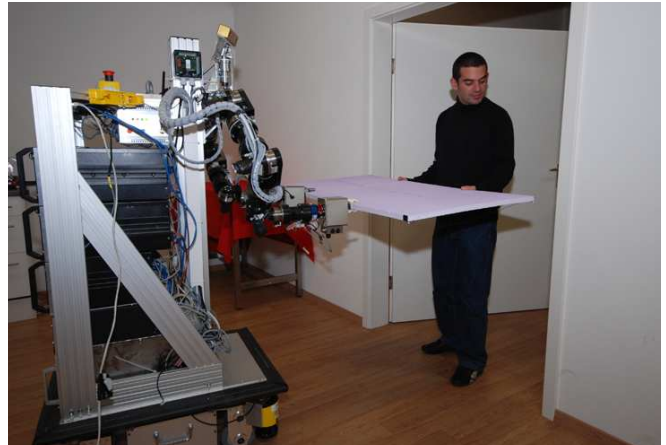
Fig. 1. Envisaged scenario of a joint load transport: Human and robot cooperatively carry a bulky object through a constrained environment.
