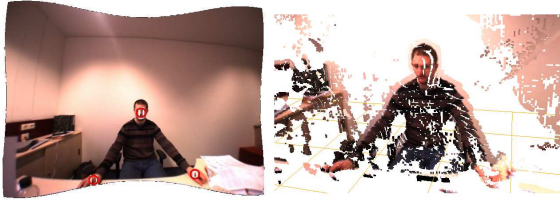
Fig. 7. Image with detected skin parts (left). This image has been taken with a stereo camera with a high aperture and has already been rectified. The right side shows the three-dimensional reconstruction of the scene using a stereo matching algorithm.
