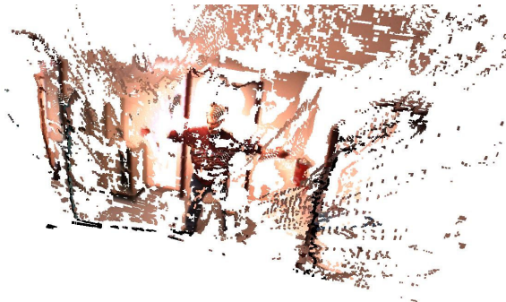
Fig. 7. Colored point cloud from the stereo vision algorithm
