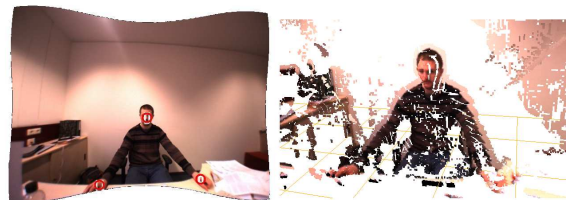
Fig. 3. Image with detected skin parts (left). This image has been taken with a stereo camera with a high aperture and has already been rectified. The right side shows the three-dimensional reconstruction of the scene using a stereo matching algorithm.
