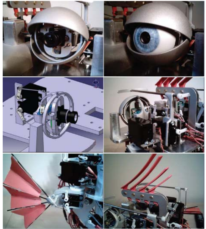
Fig. 3. Mechatronics from upper left to lower right: left eye; left eye with iris cover; CAD-drawing of right eye gimbal; eye-brow mechanics; ear mechanics; crown mechanics.
