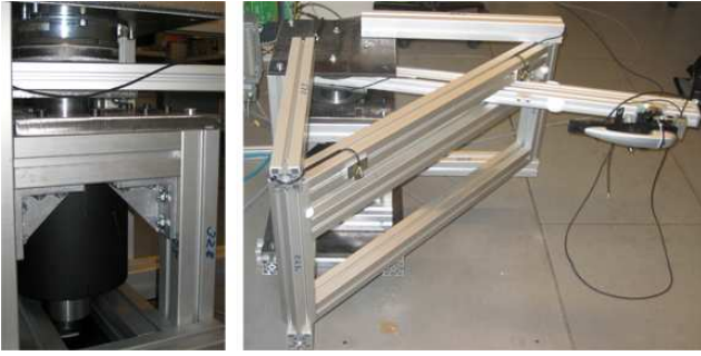
Fig. 10. Setup of the high-fidelity haptic device for car door simulations, featuring a direct drive ( \tau_{max} = 100Nm ) and an outer door handle as end-effector (l: drive, rod, and brake; r: whole setup)
